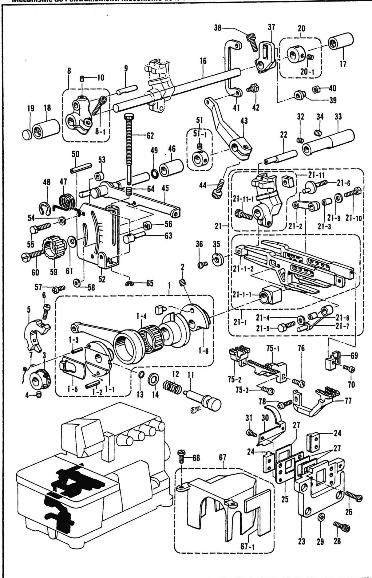
E. 送り関係 / Feed mechanism / Transportvorrichtung /
