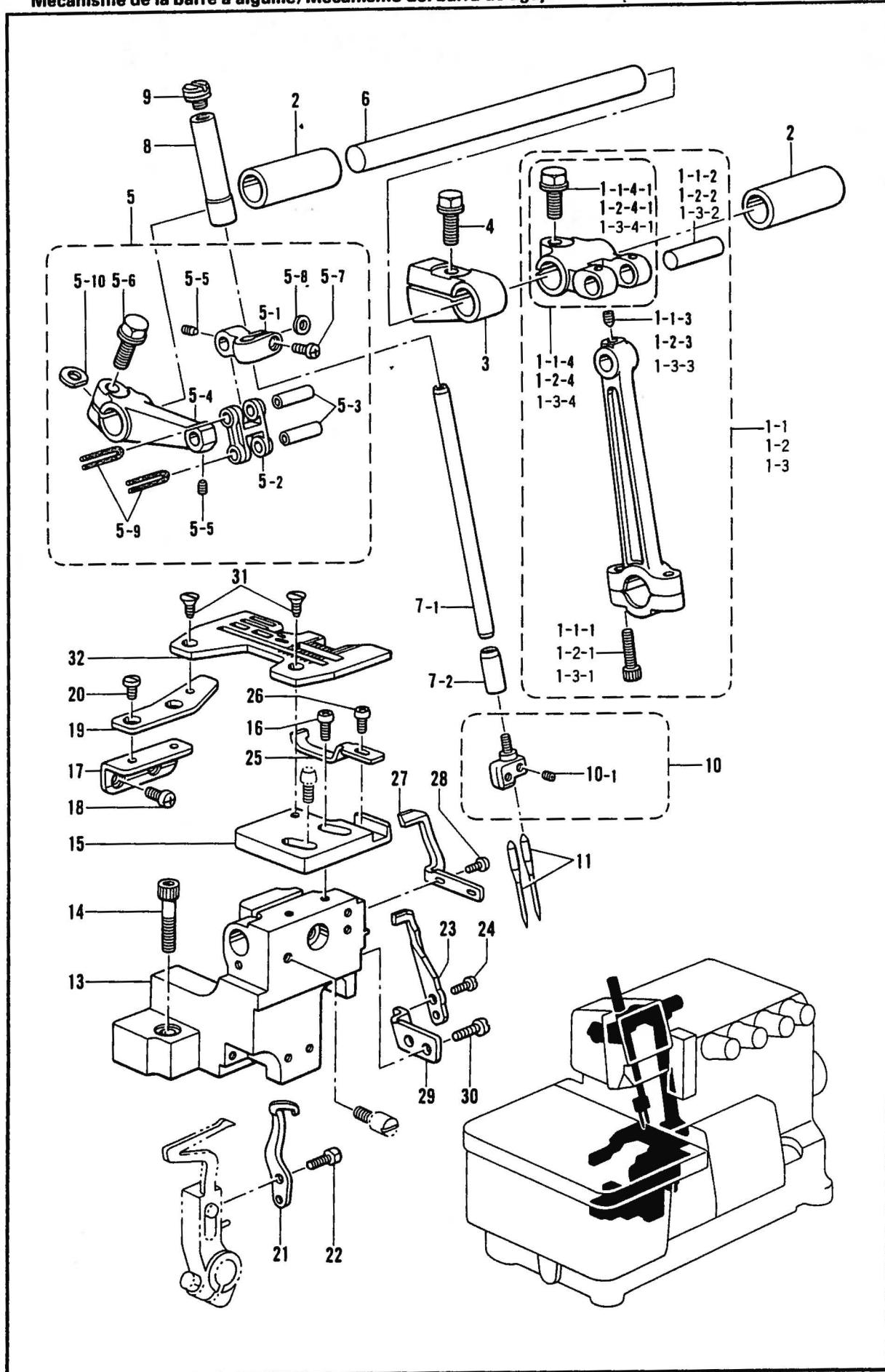
C. 針棒関係/Needle bar mechanism/Nadelstangenvorrichtung/
