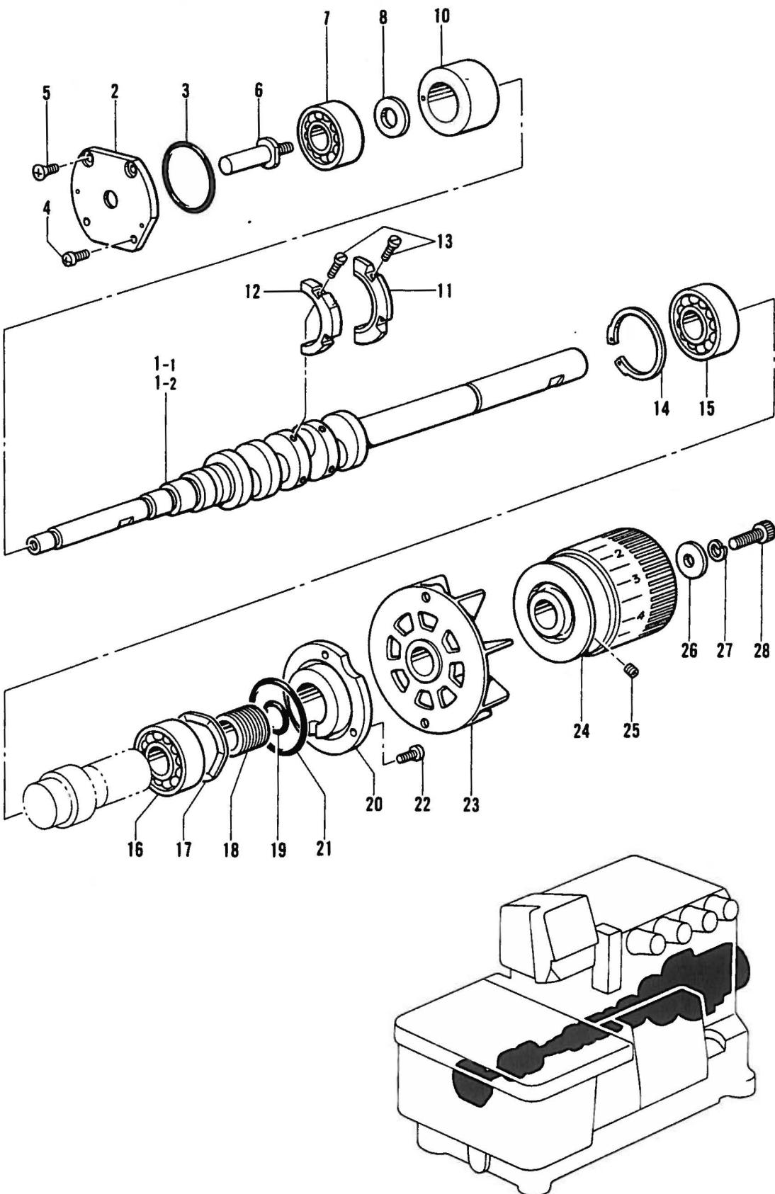
B. 駆動軸関係/Crank shaft mechanism/Kurbelwelle/
